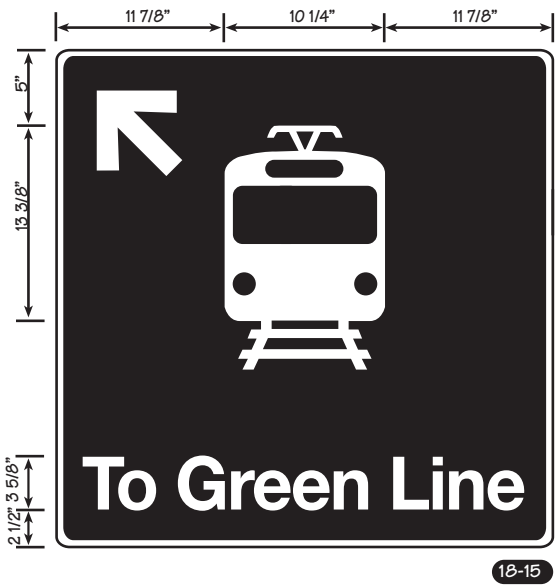
COPY LAYOUTS (SHOWN HERE FOR FLUSH MOUNTED APPLICATION) SCALE: NT5
